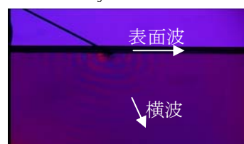
Fig.5. Visualized elastic wave pattern by sensitive method.
