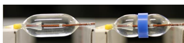
Fig. 2 Comparisons of balloons with/without a ring. Each one expanded with 17 mL of water.
